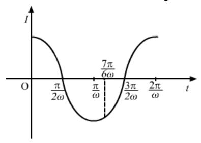
As shown in the figure, from t=0 to  $\frac{7\pi}{6\omega}$  the charge will be maximum at  $t=\frac{\pi}{2\omega}$ , when current in the circuit is zero.
