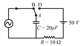
(A) Magnitude of the maximum charge on the capacitor before  $t = \frac{7 \text{ K}}{6\omega}$  is  $1 \times 10^{-3} \text{ C}$
